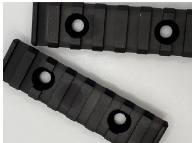
Blast shadowing is a common challenge that occurs when features of the component shield or mask blast media access. Inconsistent surface texture results in visual inconsistencies.
