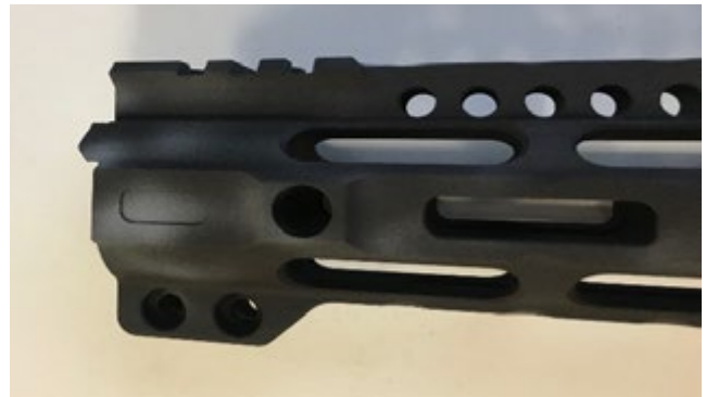
Inconsistent blasting is a common defect associated with manual blasting. Over-blasting – using too much pressure, not enough travel, and extended dwell time – produced the defect shown above. Prior to hard anodizing the issue was almost undetectable.
