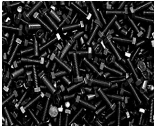
Black oxide or 'bluing' is commonly used in ferrous substrate components such as fasteners, brackets, and even frames or receivers.
